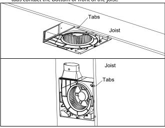
2. The housing mounts with 4 screws (Ø4×25 mm). Screw housing to joist through the round holes in each mounting flange, then through the other holes.
