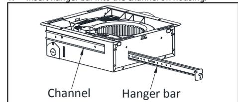
2. The flange of housing mounts with two tapping screws (Ø 4x25 mm). Fasten hanger bar to joist with two tapping screws (Ø 4x25 mm) and secure it to joist with machine screw (# 8-32x5/16").
