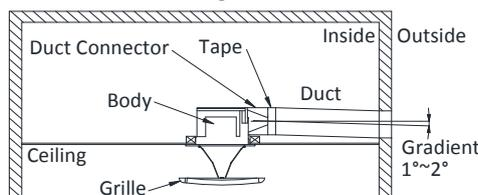
**CONNECTION METHOD FOR 3" ROUND DUCT CONNECTOR**
