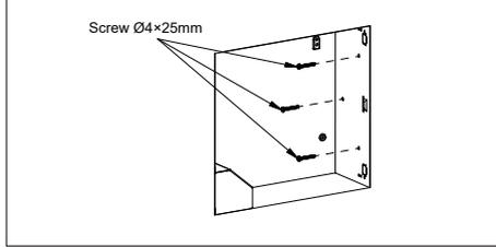
5. Do the duct work as below picture and follow "DUCT CONNECTION" and then fix the duct connector to the housing inside by using machine screw (M4 x 6 mm).
