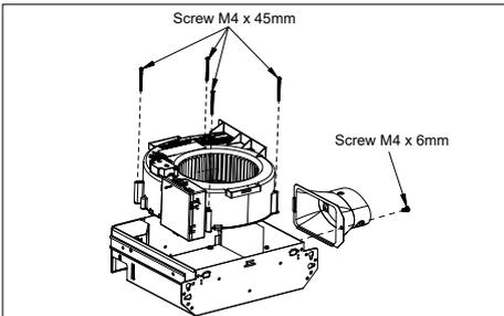
4. Using wire nuts (not provided) connect house wires to fan wires as shown in "CONNECT WIRING" diagram A. Insert housing into ceiling or wall opening and secure housing by using tapping screws (ø 4x25 mm).
