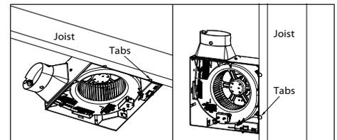
2. The housing mounts with 4 screws (Ø4x25 mm). Screw housing to joist through the round holes in each mounting flange, then through the other holes.
