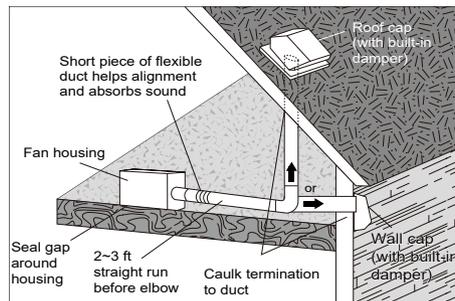
Proper insulation around the fan to minimize building heat loss and gain. The ducting from this fan to the outside of the building has a strong effect on the air flow, noise and energy use of the fan. Use the shortest, straightest duct routing possible for best performance, and avoid installing the fan with smaller ducts than recommended. Insulation around the ducts can reduce energy loss and inhibit mold growth. Fans installed with existing ducts may not achieve their rated air flow.
