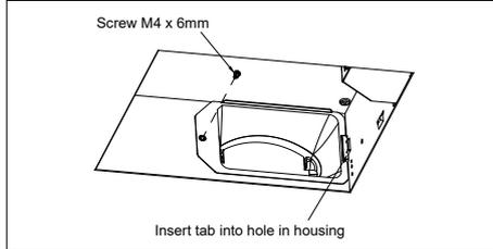
6. Insert fan body into housing by using four machine screws (M4 x 45 mm) originally on the fan body and plug in all connectors.
