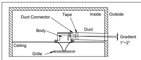
Connection method for 3" round duct connector
