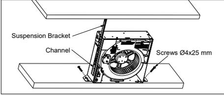
3. Extend suspension bracket to the width of the joists. Make sure the fan body is level and perpendicular with the joist, and flush with ceiling surface.
