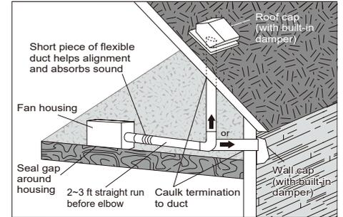
Proper insulation around the fan to minimize building heat loss and gain. The ducting from this fan to the outside of the building has a strong effect on the air flow, noise and energy use of the fan.
