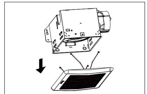
2. Remove dust and dirt from the fan body with a vacuum cleaner.
