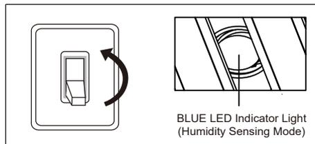
Full Speed Mode: Cycle ON/OFF fan switch to operate at full speed mode. The LED indicator light will be AMBER.
