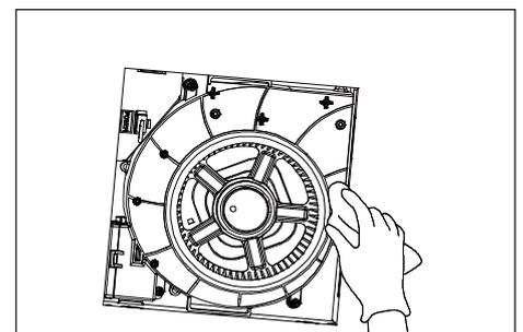
4. Replace the grille back onto the fan body.
