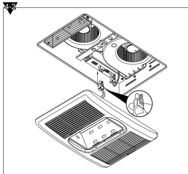
c. Install the Grille Assembly **2** into the Fan Body **1** using the Machine Screw **B**.
