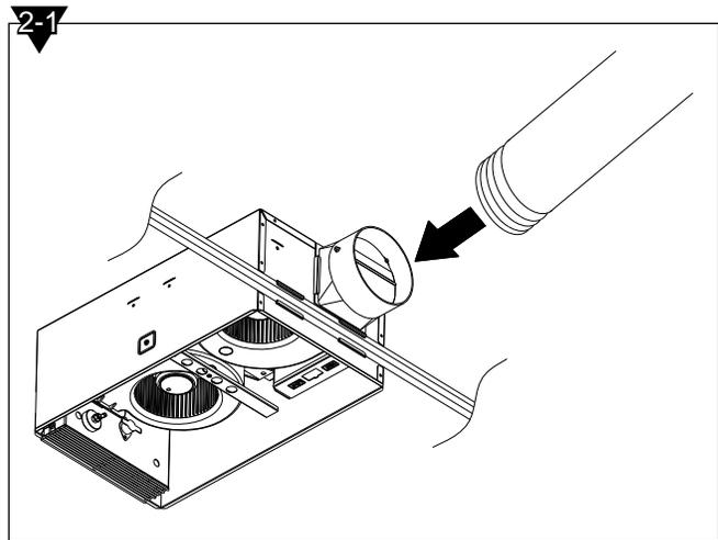
b. Do not install the unit where ducts are configured as shown in Figure 2-2. Install the duct with a gradient of 1°-2° to the outside.
