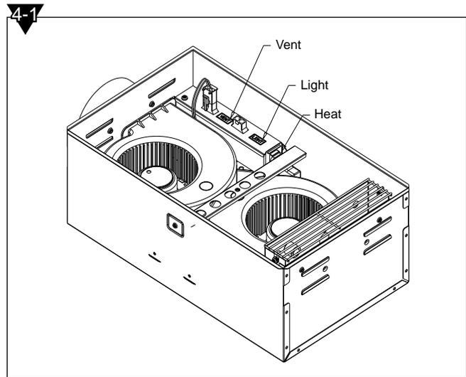
b. Plug the Light Connector into the receptacle marked "Light"
