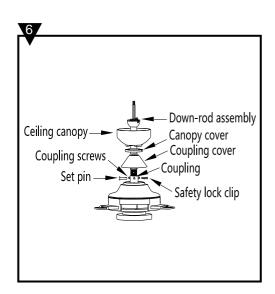
2. (Fig. 7) Install down-rod into motor housing coupling, aligning the holes and install set pin and safety lock clip. Insert set pin through coupling and down-rod until point appears on the other side, and insert safety lock clip on set pin. Pull the down-rod up tight against the set pin, and then evenly tighten the down-rod set screws on motor coupling. Place coupling cover on motor assembly.
