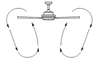
**Winter** - An upward air flow moves warm air off the ceiling.
